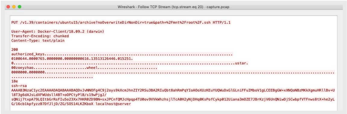
Figure 6. Putting a custom authorized key inside a mounted filesystem
