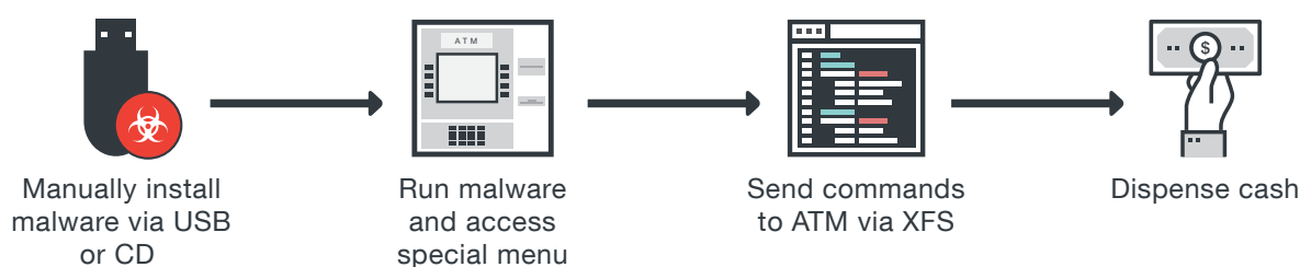
Figure 3. How a typical physical ATM malware attack is carried out
