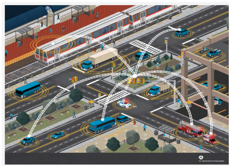
Figure 10. Vehicle-to-Vehicle (V2V), Vehicle-to-Infrastructure (V2I), and Infrastructure-to-Infrastructure (I2I) communications in future roadways
