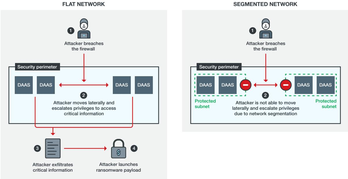
Figure 9. A diagram showcasing the differences in security between a flat network and a segmented network
