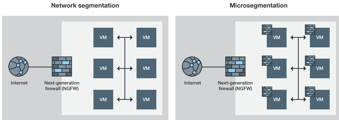
Figure 10. A diagram showcasing the differences between network segmentation and micro-segmentation
