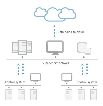
FIGURE 1: Sample internally hosted SCADA application where data is externally pushed
