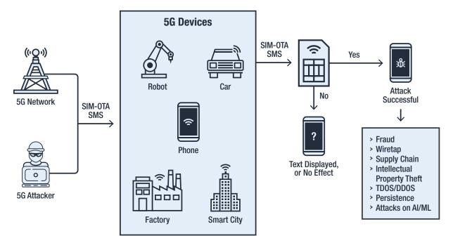
Figure 3. A visualization showing SIM jacking by abusing the SIM-OTA SMS operational technology (OT)
