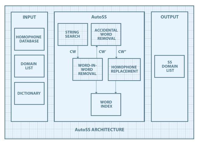
Figure 1: AutoSS's architecture; given a homophone database, a list of target domains, and a dictionary, AutoSS outputs a list of possible soundsquatted domains
