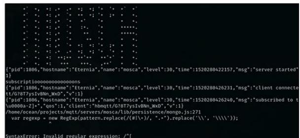
Figure 15. Result of CVE-2018-11615 exploitation against Mosca, a popular MQTT broker.
