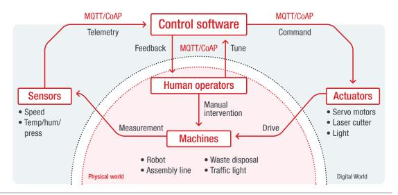
Figure 47. Abstract IIoT scenario with sensors producing data, actuators receiving commands, and control software, operators, and other roles
