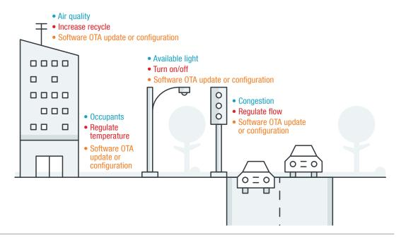
Figure 57. Abstract smart city scenario. As in the smart-factory case, each node serves three functionalities: actively affect the physical world, measure from the environment, and be an IT node to be managed.
