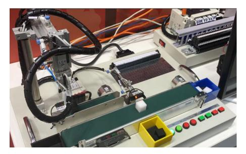
Figure 49. Prototype, small-scale production line that Trend Micro built for explaining and demonstrating security risks to its customers
