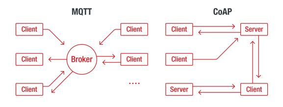
Figure 1. High-level view of the interaction models of MQTT (left) and CoAP (right)
