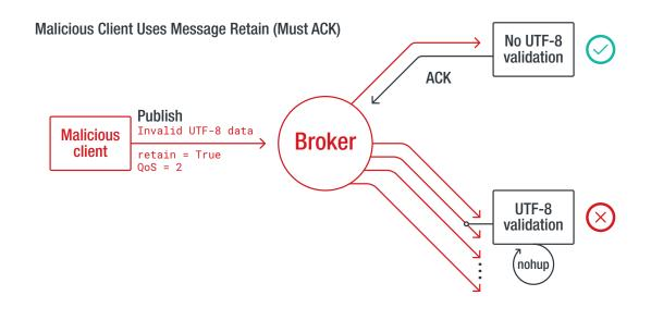
Figure 10. A malicious client could exploit the discrepancy between validating versus non-validating nodes to keep nodes offline. Surprisingly, in this case, not following the standard is the best approach for a client.
