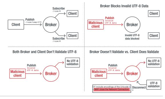
Figure 9. Context (top left); a broker that implements the check as in the standard (top right); both client and broker do not implement the check (bottom left); the broker lets invalid character pass, while the client follows the standard (bottom right).
