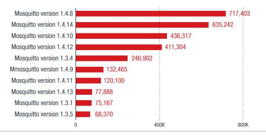
Figure 14. Breakdown of the top 10 most popular MQTT broker versions according to our internet-wide scan data analysis. Notice that the most current Mosquitto versions, 1.4.15 and 1.5, are not among the top 10. All of the top deployments of Mosquitto are vulnerable (including 1.4.15).
