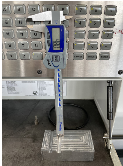
Figure 19. The defective engraving as shown by the caliper
