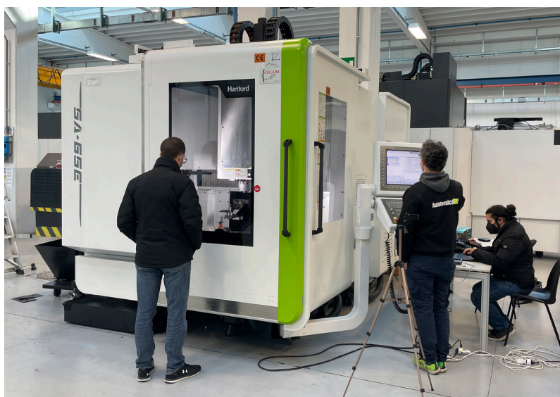
Figure 12. The Hartford 5A-65E machine, running on a Heidenhain TNC 640 controller, that we used in our experiments at Celada
