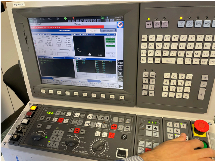
Figure 10. The Okuma simulator we used for the development of the malicious application and during the initial testing
