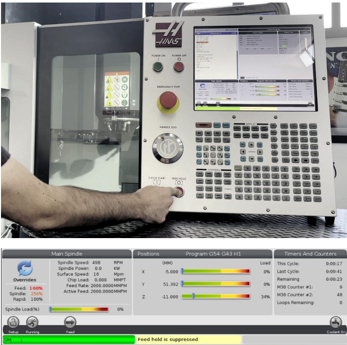
Figure 15. A demonstration of the “disabling feed hold” attack: the operator pushing the feed hold button to no effect (top) and the details of the console (bottom)
