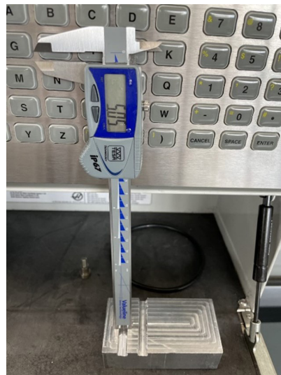
Figure 17. The correct engraving measurement as indicated by the caliper
