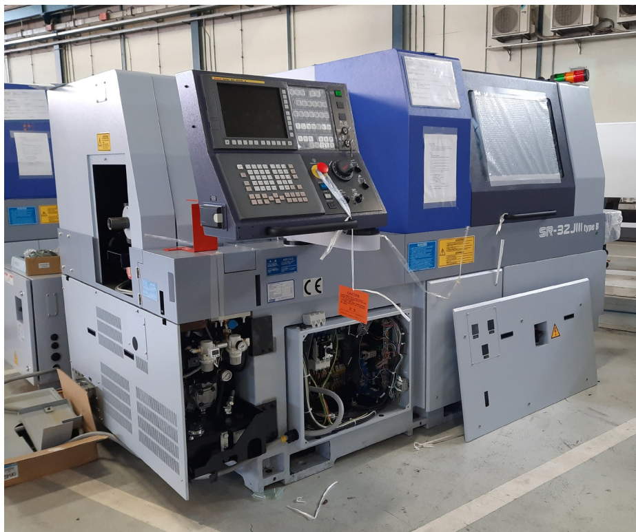
Figure 14. The Star SR-32JII machine, running on a Fanuc controller, that we used in our experiments at Celada
