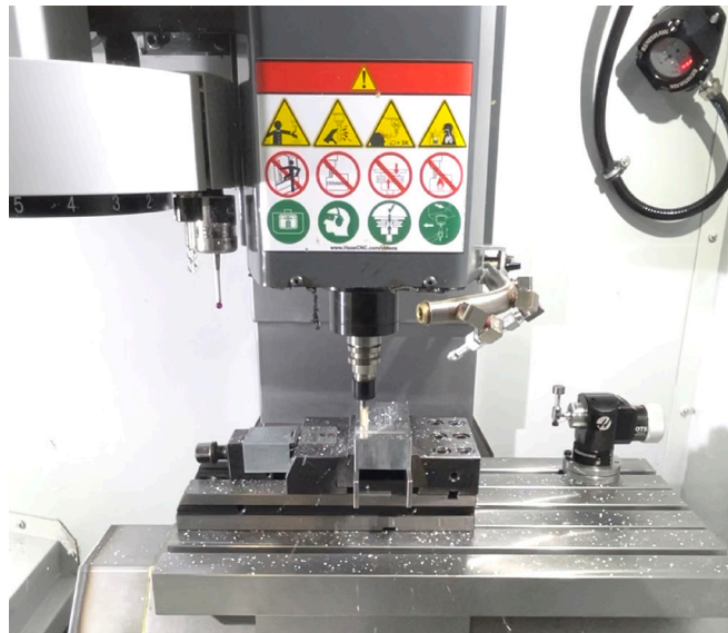
Figure 16. The Haas Super Mini Mill engraving trace number 2 during our experiment
