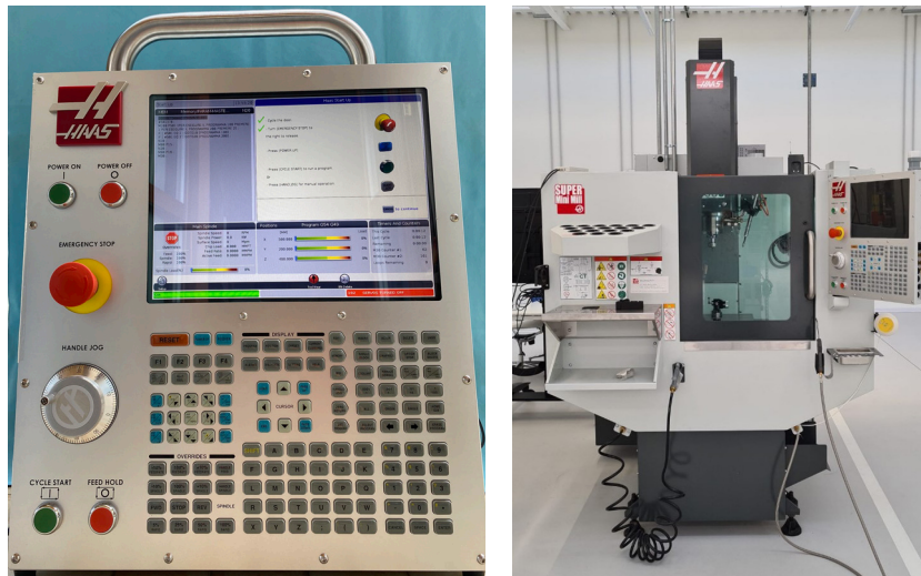
Figure 8. The Haas simulator we used for preliminary testing (left) and the Haas CNC machine (Super Mini Mill 2) by Celada we used for verification (right)
