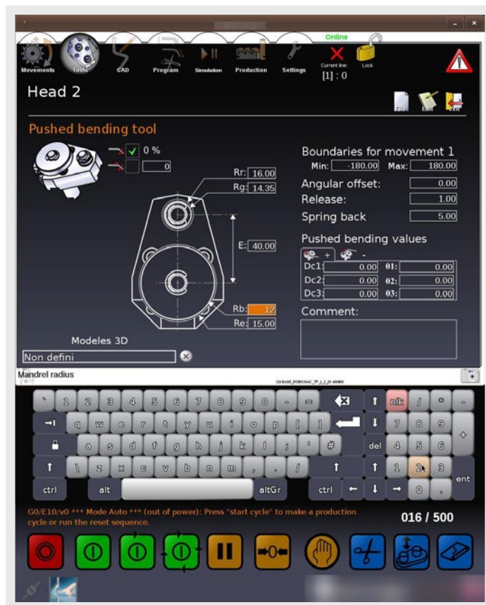
Figure 15. Exposed HMI for a bending tool
