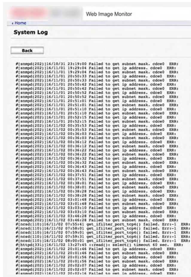
Figure 17. A screenshot of the system log and network information from an exposed printer
