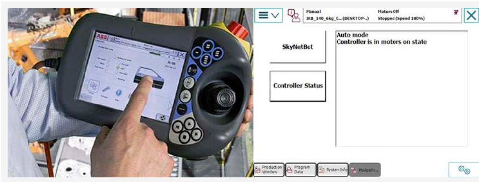
Figure 21. Left: HRI screen used to manually control the movements of a robot's arm from abb.com; right: modified HRI screen showing that the robot is in “motor off” (or “manual mode”) when it is in “auto” (or “motor on”) mode, which means it will not respond to manual commands issued through the HRI joystick
