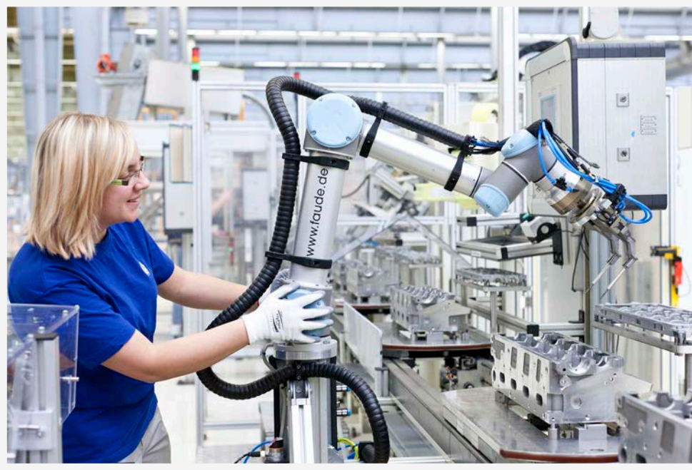
Figure 3. Co-bot working closely with a human operator with no physical safety measures
