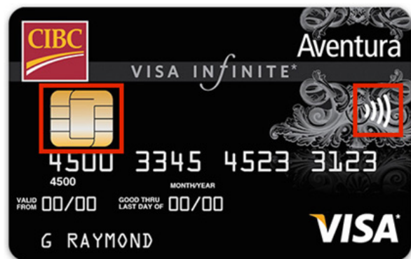
Figure 51: CIBC credit card that uses the EMV and RFID technologies
