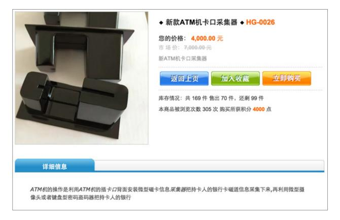
*Figure 13:* ATM skimmers cost RMB 4,000 (~US\$631) each; these came installed with a microchip that records payment card track data or the confidential information stored on a card's magnetic strip, along with a microcamera that allows cybercriminals to obtain a victim's PIN
