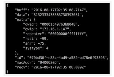
Figure 15. MQTT message for payload transmitted over LoRa
