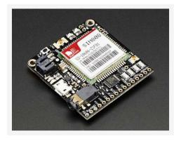
Figure 14. A SIM808 module (Source: https://www.adafruit.com/product/2542)
