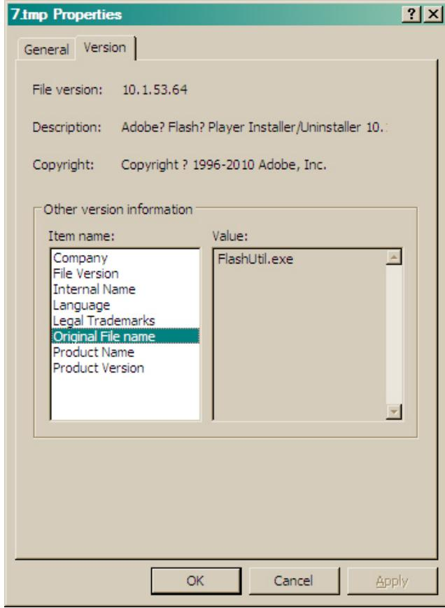
**Figure 1.** File properties of the .TMP of the malicious executable file
