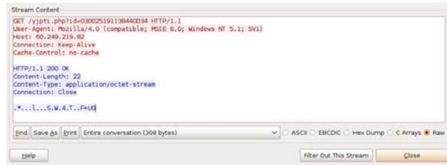
**Figure 3.** Network communication between a Taidoor compromised machine and a Taidoor C&C server
