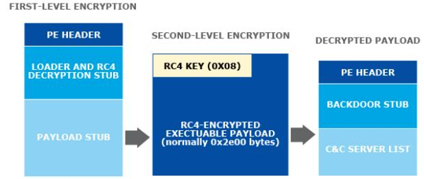
**Figure 2.** File structure of encrypted SIMBOT malware variants
